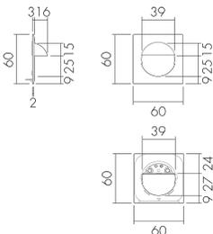
Abmessungen in mm
