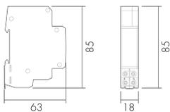
Abmessungen in mm
