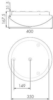
Abmessungen in mm
