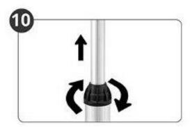
Adjust the height requested with tightness of plastic colar.
