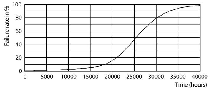
Lumen Maintenance Diagram - MAS LED spot VLE DT 6.2-80W GU10 927 36D
