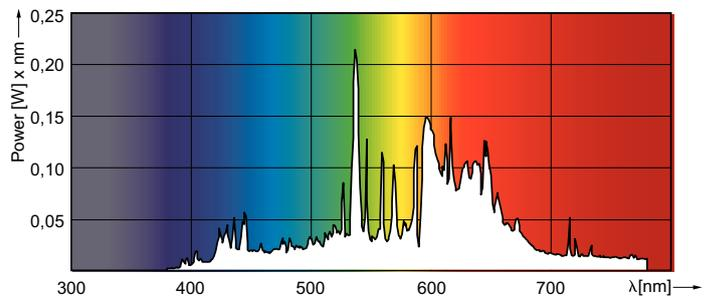
Spectral Power Distribution Colour - MC CDM-R Elite 35W/930 E27 PAR30L 30D
