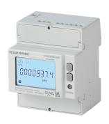
The COUNTIS E4x is a modular electrical energy meter displaying the energy (kWh, kVArh and kVA) and other measurements directly on its backlit LCD display. It is designed for three-phase load metering with connection via CT and is suitable for applications of up to 12000 A.
