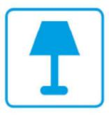
This luminaire contains built-in LED lamps
