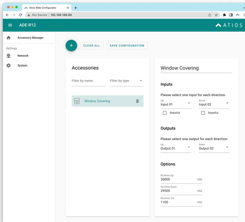
The motor directions UP and DOWN can be inverted by switching the outputs, vice versa for the inputs.
