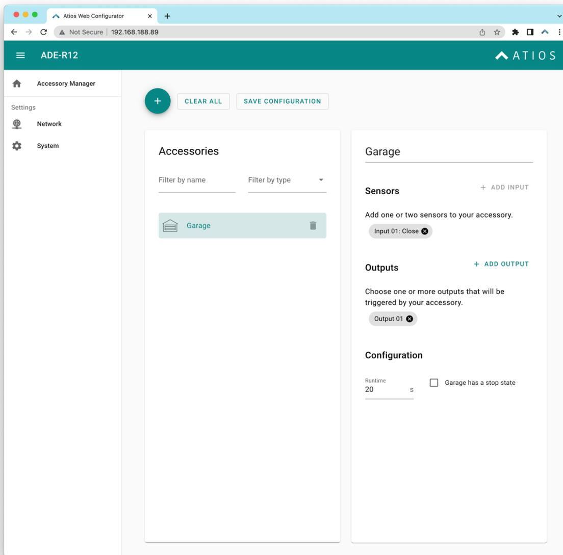
Multiple Door sensors (one for Closed, one for Open) will be supported soon. Until then please use the runtime option, and fill in the time in seconds that the Garage needs to completely open.
