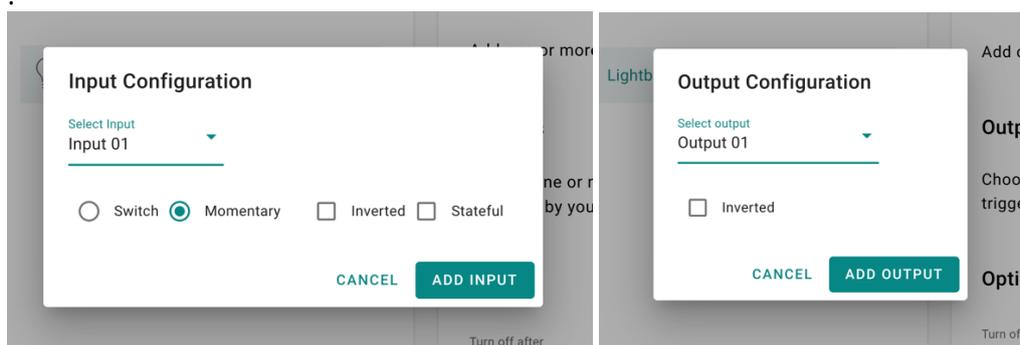
One input can be assigned to multiple outputs, as well as multiple outputs to a single accessory. A Switch, an Outlet and a Valve are configured similarly.
