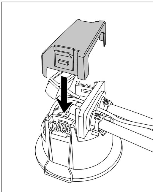
7. Insert the device with the mounting folded up into the installation opening.
