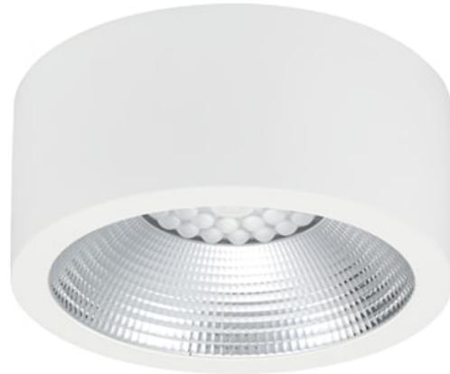
Insaver is a surface mounted LED downlight ,Die-cast aluminium body, loop in loop out connector for quick installation, Non dimmable LED driver, 20W; 2350lm; 118lm/W; 3000K; UGR <19 with height of 95 mm. Meets TP(a) requirements.
