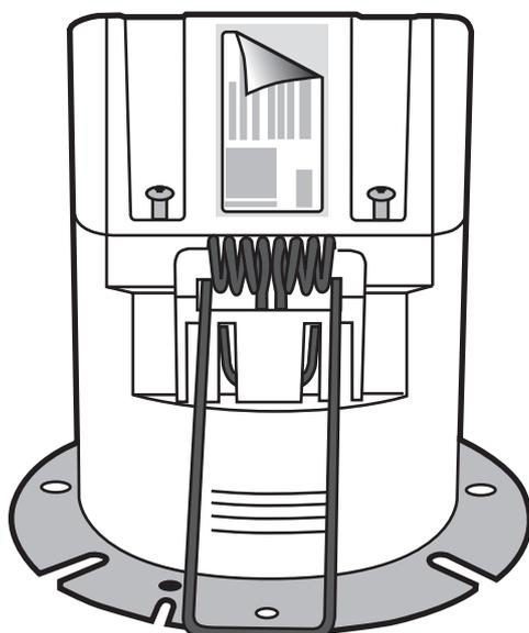
2. Insert the device - with the mounting springs folded up - into the installation opening.
