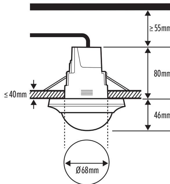
The required clearance above the Powerbox depends on the bending radius of the installation cables (example: 55 mm).
