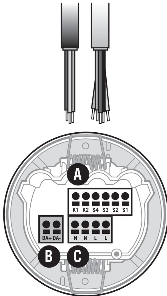
5. If necessary, route a protective earth conductor via a separate terminal.
