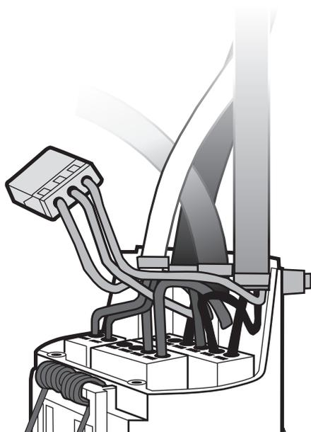
6. Use the included cable ties to secure the cables to the Powerbox for strain relief.
