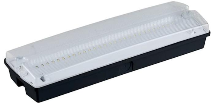
LiFeSafe PRO BH IP65 C EM3 NM/MT DA BLK is a black DALI addressable LED surface or recessed LED bulkhead. Black steel recessing kit available as an accessory. Maintained or Non-Maintained, 3Hr emergency duration, complete with 4 ISO7010 Exit legends, Left, Right, Up and Down. Maximum viewing distance 30m. 0 to +45°C operating temperature range. IK10, IP65, Class II electrical construction, 6-year warranty.
