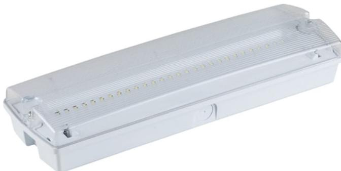
LiFeSafe PRO BH IP65 C EM3 NM/MT DA is a DALI addressable LED surface or recessed LED bulkhead. Steel recessing kit available as an accessory. Maintained or Non-Maintained, 3Hr emergency duration, complete with 4 ISO7010 Exit legends, Left, Right, Up and Down. Maximum viewing distance 30m. 0 to +45°C operating temperature range. IK10, IP65, Class II electrical construction, 6-year warranty.
