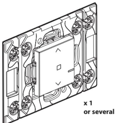
Connected switch for rolling shutters
