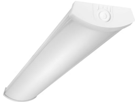
DELTAWING 1200 4K SSC is a ceiling and wall surface, suspended LED luminaire with opal diffuser, 1160x160x60mm dimensions, 36W system power, 4,600lm flux and 128lm/W efficacy, CRI (Ra) >80, 4000K (Neutral White) CCT, chromaticity tolerance of 3-step MacAdam ellipse, SylSmart Standalone enabled, RAL9003 finishing, L70B50 100khrs / L80B50 80khrs lifespan, IK06 impact resistance, IP44 ingress protection rating (in ceiling surface installation), Electrical protection Class I, Glow wire test 850°C.
