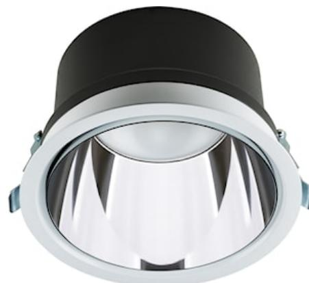
The Solstice 150 1200lm 930 DALI is a high efficient DALI dimmable downlight luminaire, Colour rendering index Ra>90, Colour temperature: 3000K Warm White, Class II, Protection rating IP40/IP20, Cut out dimensions: 150mm.
