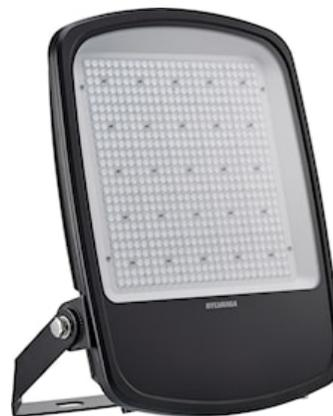
Exterior LED Floodlight, comes complete with 1000mm flying lead and adjustable bracket, aluminium housing, clear glass diffuser, integrated anti-condensation valve, IP66, IK08, Class I, 4000K, CRI80, Non-dimmable, 46400lm, 297W, 156lm/W, Symmetrical Wide beam, 100.000hrs L80B50 lifespan, 532 x 407 x 97mm (LxWxD) dimensions, 7.4kg weight, RAL9017 Traffic Black color, Ball-impact-resistance according to DIN57710-13 VDE 0710 13/5.81, DIN 18032-3.
