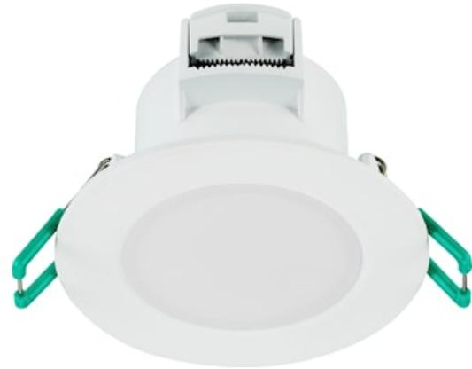
Integrated LED recessed spotlight, fixed, phase dimmable, 3 CCT 2700K-3000K-4000K, 100° degree beam angle, polycarbonate white body, low profile 47mm recessed depth, IP65 from the front, IK03, loop-in/loop-out terminals for fast wiring, 87mm bezel diameter, 68-74mm cutout, frosted lens. Additional silver or black bezel can be ordered as accessory.
